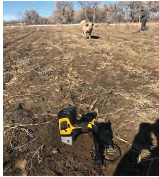
Figure 13. Portable X-ray fluorescence (PXRF) spectrometry to monitor the spatial and temporal variability of nine heavy metals including Pb, As, Cu, and Cr. NMSU ASC at Farmington 2020.
